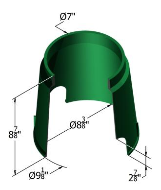
T Cover Style: HDPE Material: Model: 7" Dia. Weight: < 1 lbs Std. Fasteners: Snap-On Options: Logos and Special Markings Surface: Skid Resistant & Marked\* Performance: Pedestrian, ASTM C857, WUC 3.6,
